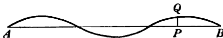
Fig. 31. The curve formed by a string performing one vibration alone is always a simple harmonic curve.
